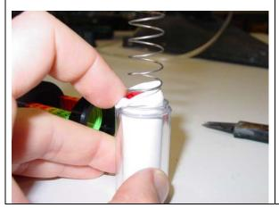
Roll the entire end of the rubber diaphragm over the outside of the clear tube and into the groove. Insert the assembly into the gauge body ensuring the snap ring locks back into the original groove.
